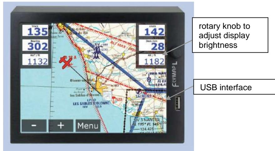
Display brightness can be adjusted by the rotary knob located on the right front side of the display casing. An USB interface for data transfer (planned flights, Flight Logbook entries, flight logs, weather data, chart/system updates, etc.) via USB memory stick is located below the rotary knob.
