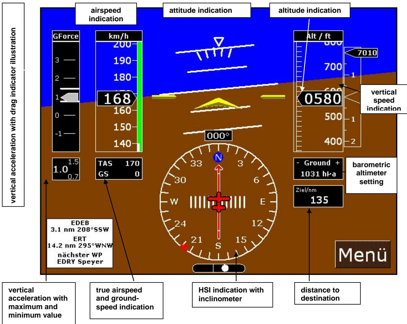
The touch-screen is also available in the PFD mode of the FLYMAP L system and can be used to center the horizon prior to beginning a flight. The barometric altimeter setting may also, for example, be selected by touching the “+” or “-” in the respective view box.
