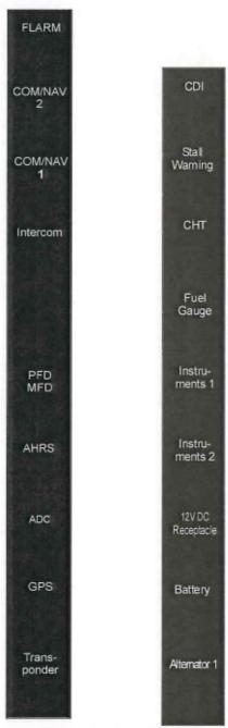
Depending on the equipment installed in the aircraft, not every position shown above might be actually assigned with a circuit breaker. In those cases the respective positions are covered by a blank plastic plug and reserved for that application by the placard.
